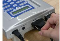
1. Connect power cord and applicators to the top end of the control unit.
