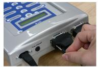
1. Connect power cord and applicators to the top end of the control unit.
